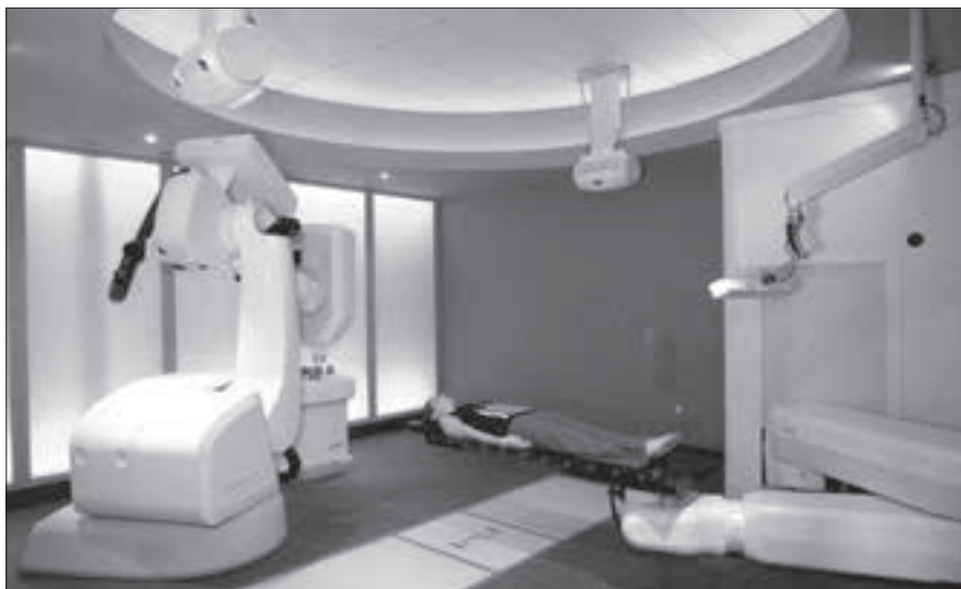
FIGURE 1: The CyberKnife LINAC is mounted on a robotic arm with six joints. One of the flat-panel amorphous silicon detectors can be seen on the side of the treatment table. (Courtesy of Accuray.com )
